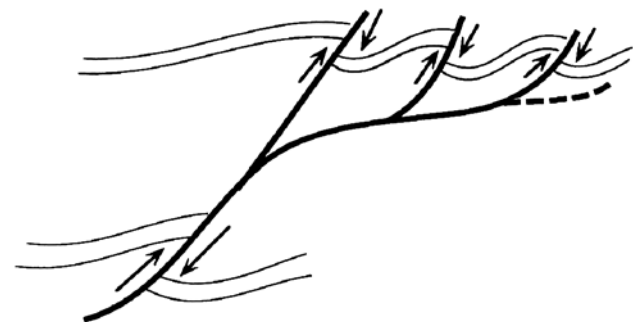
Fig. 9. A scheme illustrating near-surface widening of the fault zone with distribution of total displacement along several splitting secondary faults reaching the surface along planes of border and foothill faults, after [9, 10]. Heavy lines are faults and thin lines are sedimentary beds.
